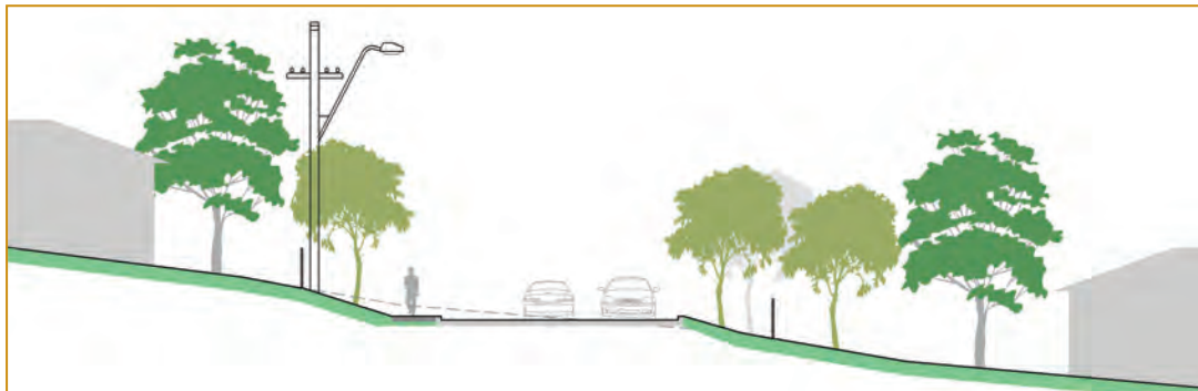
Typical cross-section of existing residential foothill street.
