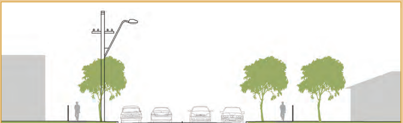
Typical cross-section of existing community link street in residential area and with on-street parking.
