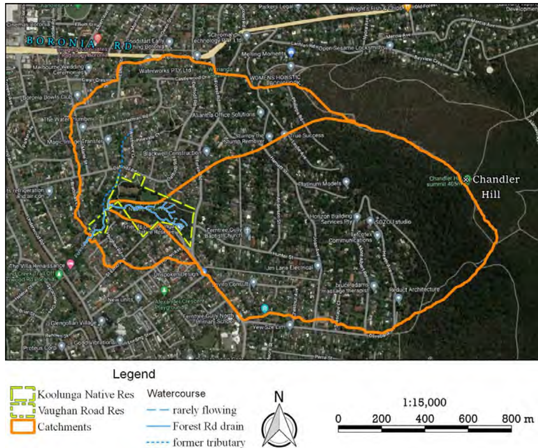
Figure 20. Catchments of Forest Rd Drain for the two reserves. The outer orange outline is for Vaughan Road Reserve. The area east of the internal orange line is the catchment for Koolunga Native Reserve.
