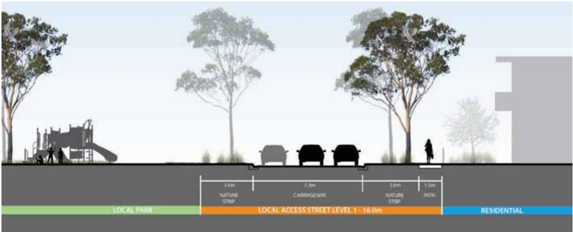
Figure 18. Local Park Interface Cross Section - Road Edge
