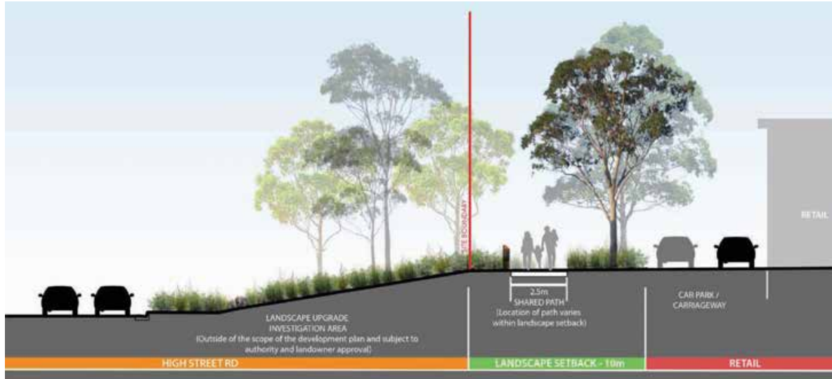
Figure 16. High Street Road Interface Cross Section - Retail
