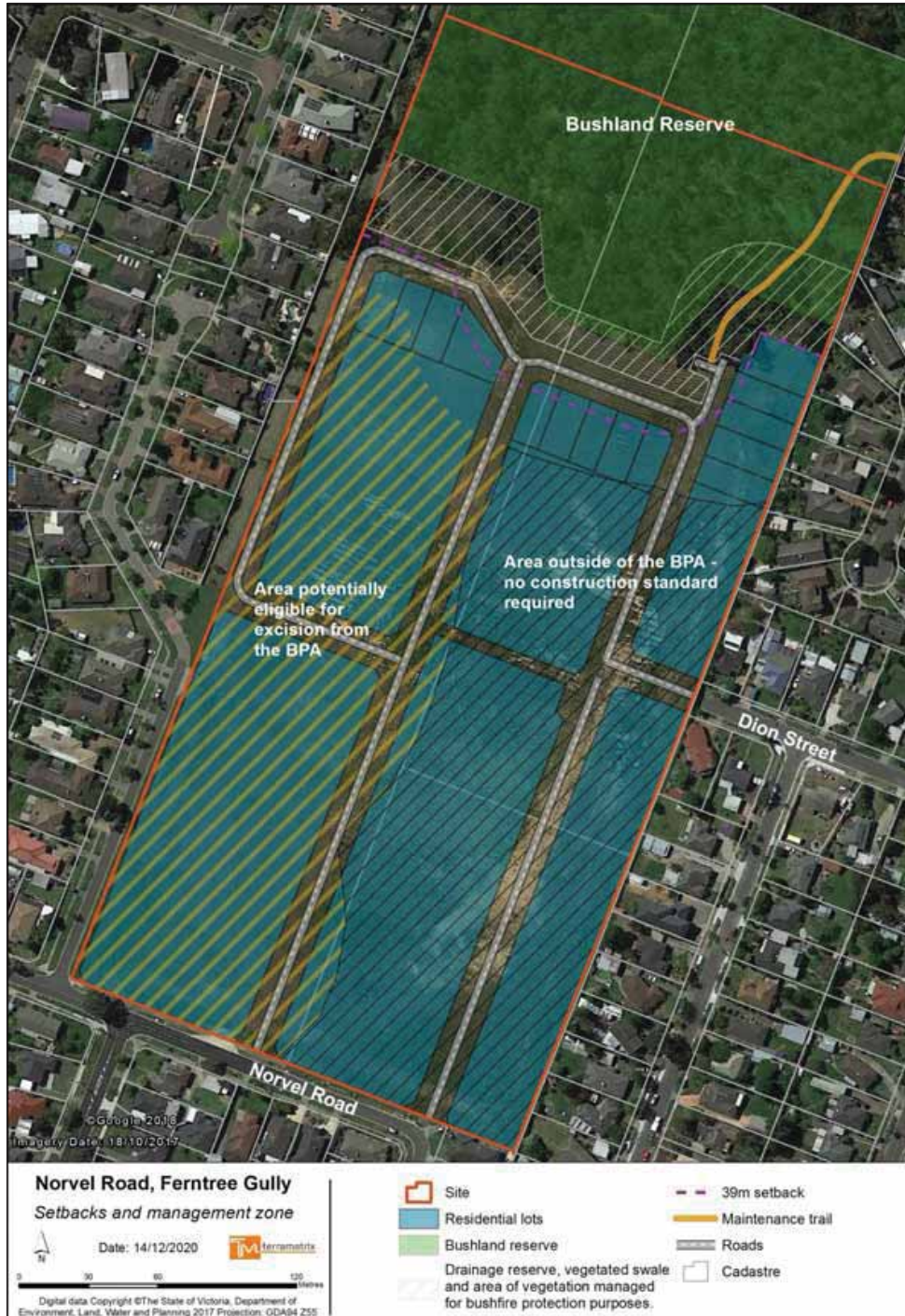
Map 4 – Setback and management zone that allow for a BAL-12.5 construction standard on affected lots.
