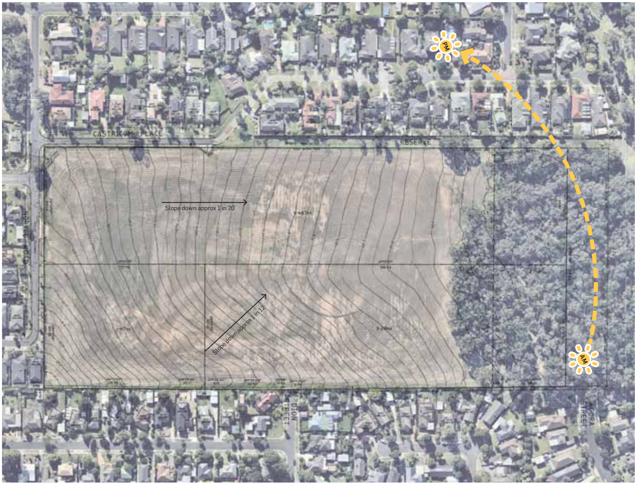
Figure 15 Site survey (Source: H.J. Macey) over aerial view
