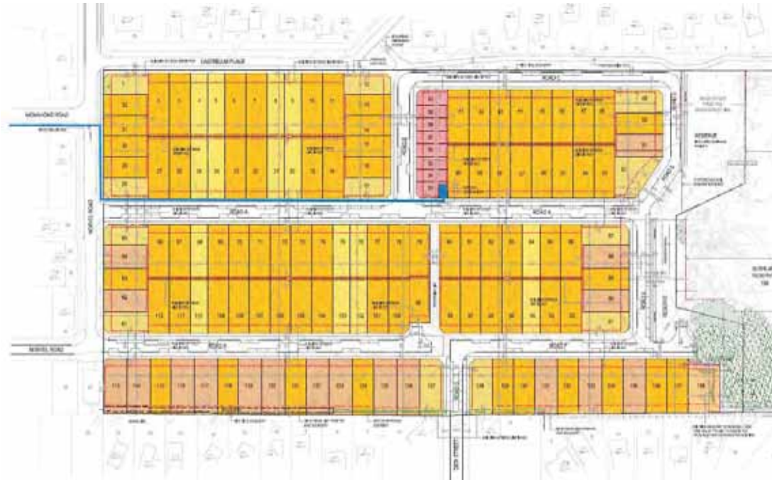
Figure 4-5 Preliminary Electrical Cable Layout
