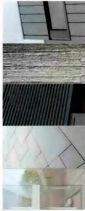
GLA 02 Shopfront Glass PAV 02 Concrete Paving LVR 02 Charcoal Colour Aluminium Louver CONC 02 Textured Precast Concrete
